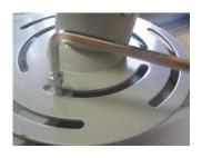
Fit the three arms as indicated on the diagram on the right hand side. When you have fitted the three arms you will then need to sit the round plate on top of the arms and move them until the ceiling mount is facing forward and towards the middle of the projector. Then move the arms until they line up with one of the slots on the mount. Then use the allen key included and tighten them up.
